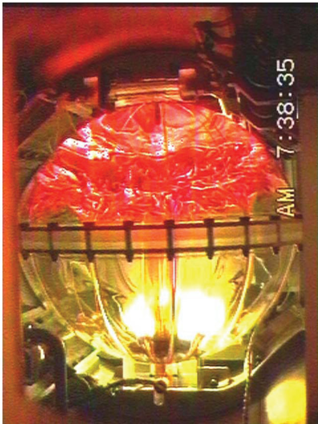
Fig. 15 Fluid position during shuttle thruster firing.
